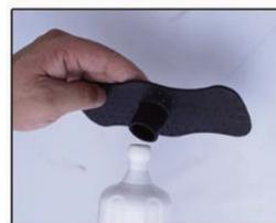
Install the base pad onto the drain cleaner.
