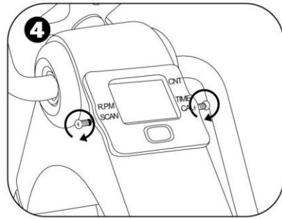
Replace the screw unit in its socket and secure with the screws.
