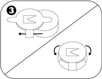
Insert a new 1,5V AG13 battery, + side down and close the tabs.
