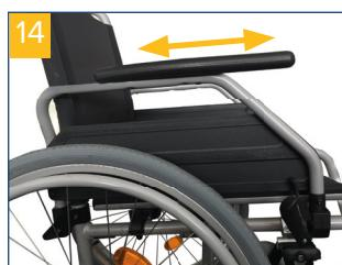
To swivel the armrest backwards, engage the release lever at the front of the arm rest and hold it down while simultaneously pulling the armrest up until the armrest is free. Now it can be swiveled backwards (**photo 15+16**).
