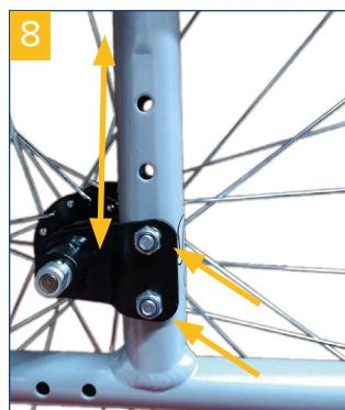
**Ensure that the wheel axle is properly tightened!**
