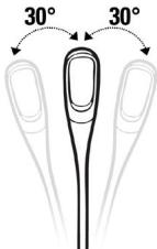
The head of the lamp can be adjusted sideways (right/left) within a 60-degree angle (30 degrees to the left and 30 degrees to the right).
