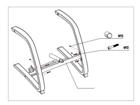
Step 3: To install seat part. Use the screw and connector to fix position which mentioned in step 2.
