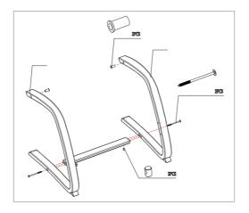
Step 2: Use the screw to fix the specified location on footrest.
