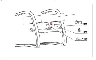
Step 4: To install backrest. Use screw to fix it together with seat part and footrest.
