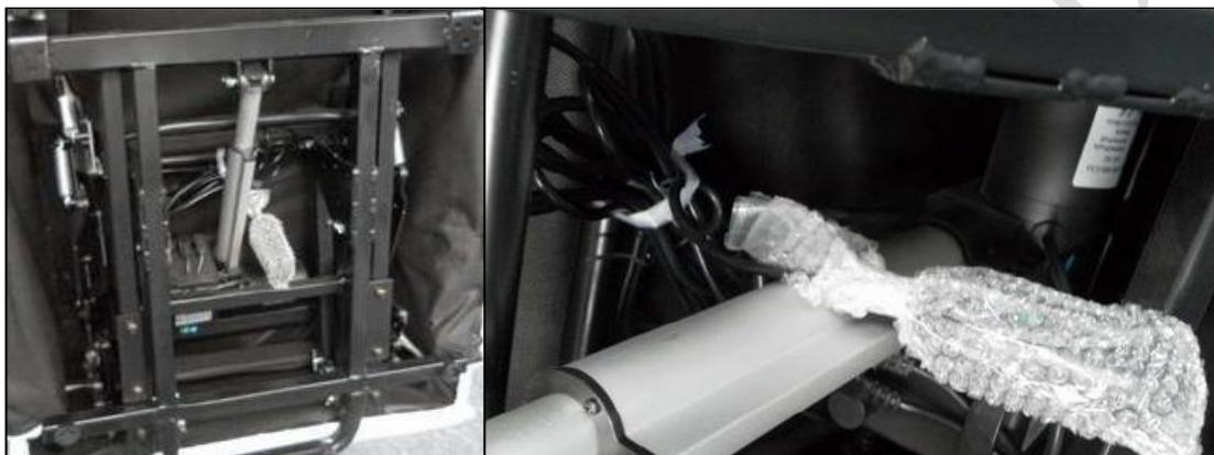
3. Pull the remote control cables out to the rear so that they cannot be pinched or damaged. For improper handling and disregard of the instructions, as well as the resulting damages, no warranty claims can be asserted!
